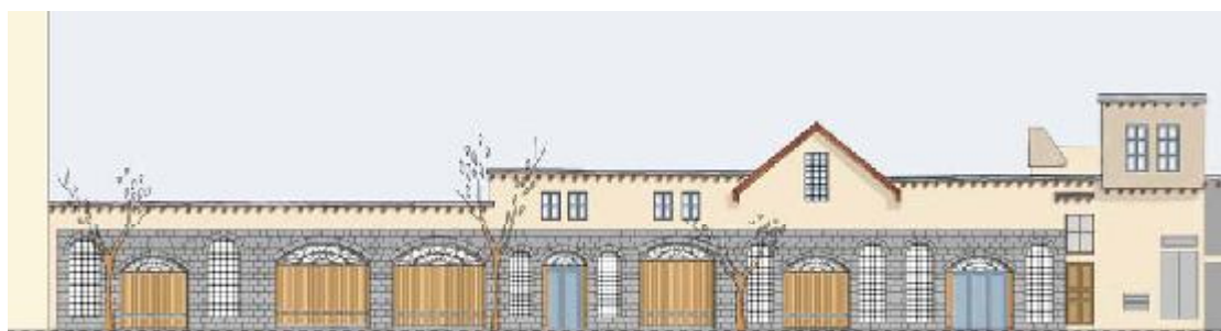
Above , a row of Ottoman-period shops and workshops on the south side of Malik Faisal Street, as existing; below , the same buildings as they would appear with later accretions removed and with the openings fitted with sideways-folding iron shutters.
