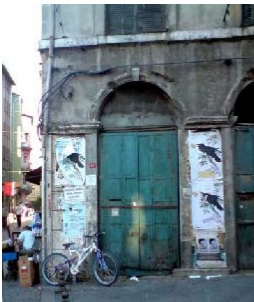
Above , pair of historic shops in Salt, Jordan. On the left, historic iron shutters leave the architecture visible, while in the case of the shop on the right, the modern face-fixed roller shutter completely conceals the arched shop front. In this case, the leaves of the iron shutters are wider than those identified elsewhere and recommended for use in Deir Ezzor.
